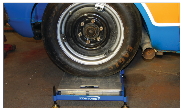
Featuring a system capacity of 6,000 lb, and an accuracy of \pm 0.1\% of applied load, Intercomp's Quik Weigh™ System is the ideal way to corner balance nearly any type of racecar.
