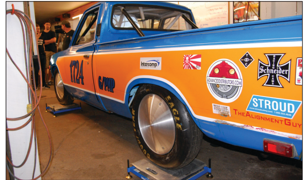
Intercomp's Quik Weigh™ RFX™ Wireless Scale System, in conjunction with standard scale levelers, are the versatile racing scales that can be easily used at any sized shop, or at the track.
